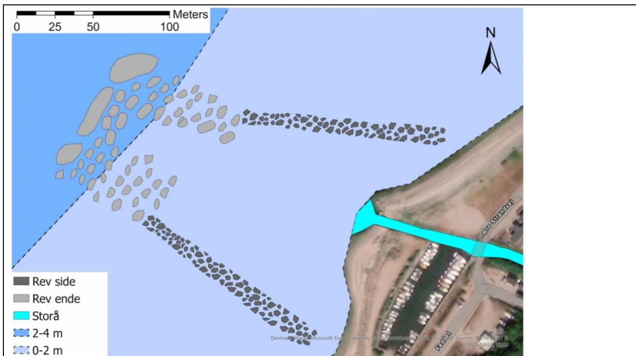
Illustration of the smolt reef by Bo Mammen Kruse (HavNatur) and Marie Hartlev Frausing (DTU Aqua). The reef is shaped like a horseshoe surrounding the river mouth.
